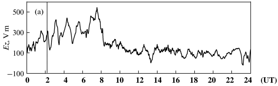
Fig. 1. Atmospheric electric field E_z in Apatity (67.3°N, 33.2°E) during SPE (ii) on 18.04.2001
